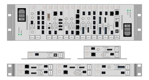
An example of Optiva's TDM capabilities are shown below. In this particular example, 12 SD-SDI video, 24 AES/EBU digital audio, 28 analog (mono) audio, 8 RS-232 serial data channels, and a 10/100 Ethernet channel are transported on just 2 fibers. CWDM could be used to combine these onto a single fiber.
