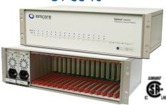
The OT-CC-6-1U series chassis is a low profile 1RU rackmount enclosure. It holds up to 6 Optiva insert cards with space for an optional SNMP Management card (Model: OPV-CTLR-IC). It features redundant, hot-swappable, fan cooled power supplies and rack reversable mountable ears. LED indicators are provided for power, fault, optical lock and network management status.
