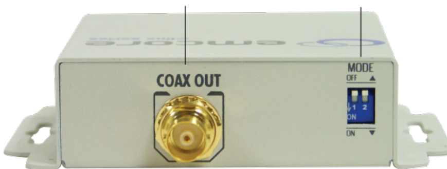
3G HD-SDI/HD-SDI/SDI Output Dip Switch ON: Firmware update mode OFF: Normal mode
