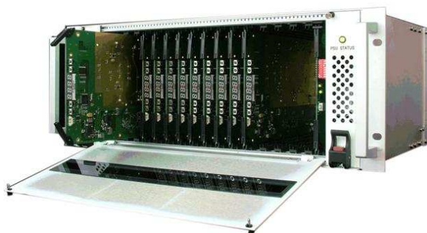
Front view showing hot-swap RF Module
