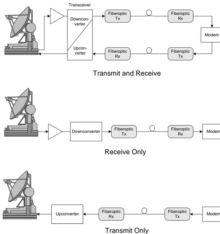
**Figure 1-1** Typical applications of the Ortel IF-band IFL.
