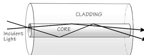
Figure 4-1 Light propagation in a step indexed fiber
