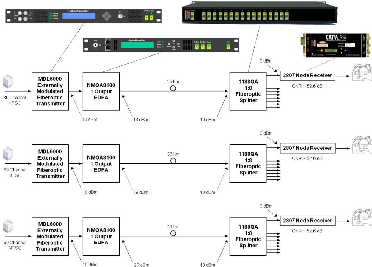
Figure 5. Distribution Network Expansion from 16 dBm to 20 dBm SBS Capability
