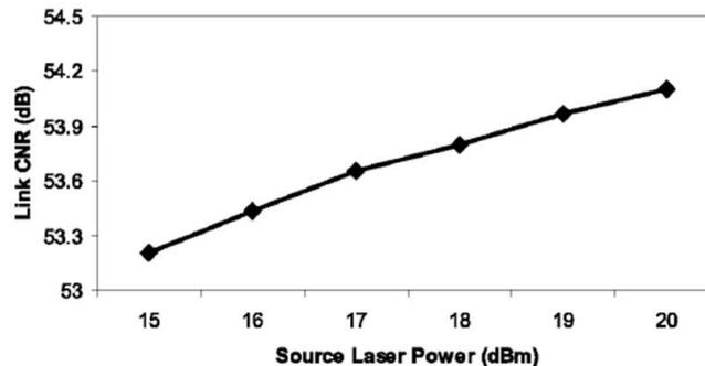
Figure 3. CNR Performance with a 17 dBm Launch-Power EDFA
