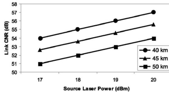
Figure 4. CNR Performance for an EDFA-less Transmitter Architecture
